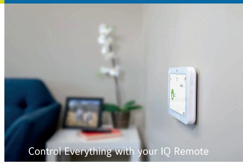
The IQ Remote is a secondary tablet that pairs with the IQ Panel 4. Not only does it provide a way to arm and disarm your IQ Panel 4 and see sensor status, but it gives you the features you don't get in your mobile app like chimes, emergency panics, and a siren. The IQ Remote can be upgraded over the air as new software upgrades are released.
